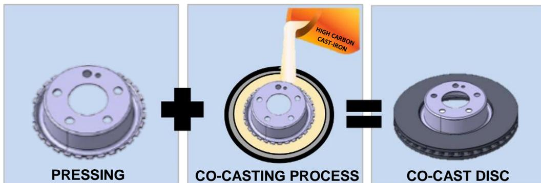
The result is a lightweight disc made up of a **high-carbon cast iron braking surface** and a **steel hat**, which are properly coupled during a special casting process that ensures perfect interchangeability with the original disc as well as **increased performance** and **reduced weight**.
